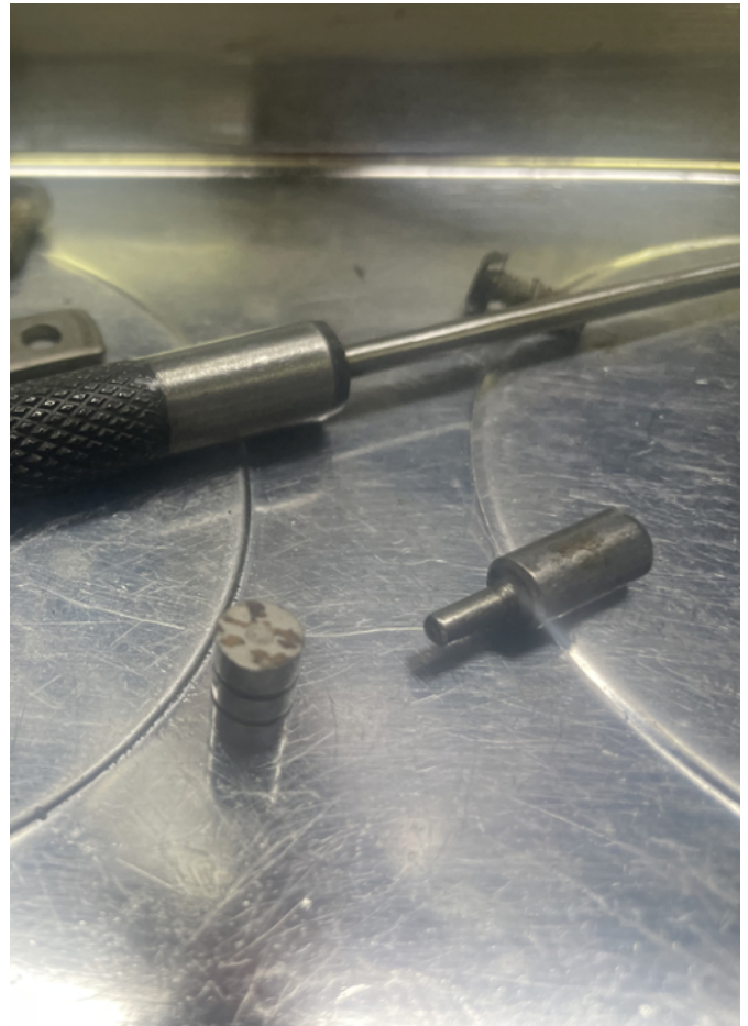
Figure 3: Rusted shuttle and end stop
